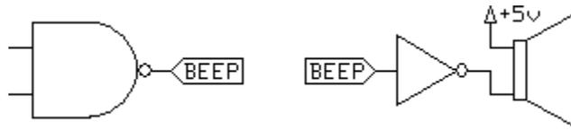
In this example, the output of the gate on the left is wired to a port symbol with the NetName *Beep*. The input to the circuit on the right (which can be on the same or a different sheet) is also wired to a port with the NetName *Beep*. This is the equivalent of running a wire between them.
