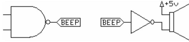
In this example, the output of the gate on the left is wired to a port symbol with the NetName *Beep*. The input to the circuit on the right (which can be on the same or a different sheet) is also wired to a port with the NetName *Beep*. The use of these two port symbols is equivalent to running a wire between them.
